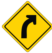
Road Curves to the Right
